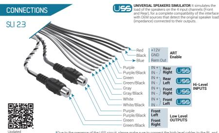
Due to the presence of the USS circuit, please make sure to connect the high level cables to the RL and RR inputs only if they are disconnected from the OEM rear speakers.
