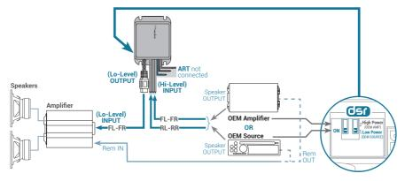
DSR: (DOUBLE STEP-DOWN RATIO) High-Power (6.5.1) and Low-Power (4.1) step down conversion ratio selectable via DIP switch independently for each input, front and rear, for a correct interface with both traditional OEM sources (Low-Power) or OEM amplifiers featuring high-voltage outputs (High-Power) up to 35V RMS.
