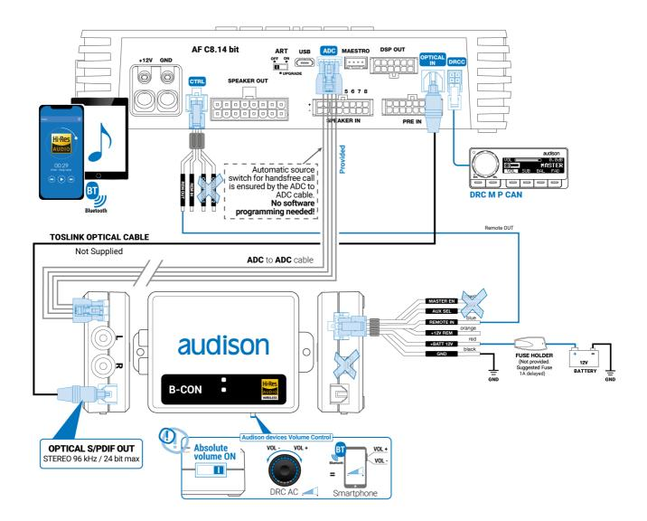
When the streaming starts from the B-CON, the main control commands of the player will be enabled on the DRC MP CAN display.
